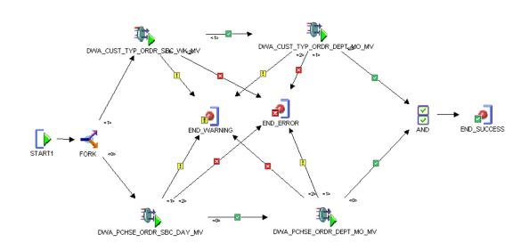
After the ORDM\_AGG\_DEP\_FLW is initiated and starts successfully the process flow moves to the Fork. The FORK process makes the aggregates to run in parallel. The AND activity specifies all the parallel aggregates must complete, then the flow switches over to the next activity, (for example, END\_SUCCESS).
