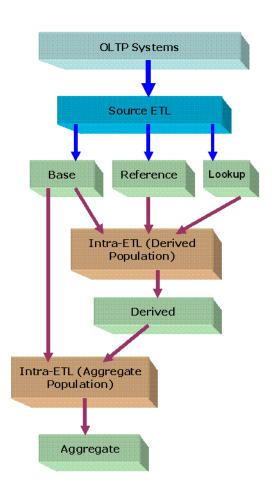
Figure 4–1 ETL Flow Diagram
