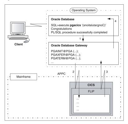
Figure 1–3 Communication Between the Oracle Database and the Mainframe, Using SNA
