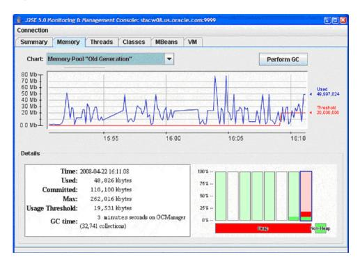
Figure 2–20 Memory Tab of the JConsole Interface When Used Memory Exceeds the Usage Threshold
