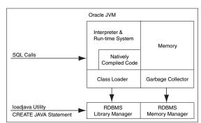
Figure 1–8 Main Components of an Oracle JVM
