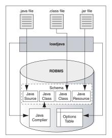
Each Java class is stored as a schema object. The name of the object is derived from the fully qualified name of the class, which includes the names of containing packages. For example, the full name of the class Handle is:
