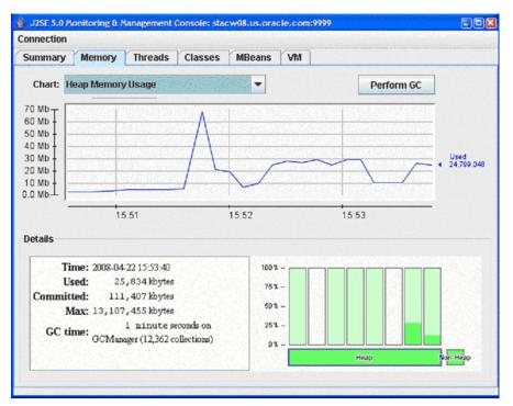
The chart on the Memory tab shows Oracle JVM memory usages versus time, for the whole memory space and also for specific memory pools. The memory pools available for Oracle JVM reflect the internal organization of Oracle JVM and correspond to object memories of Oracle JVM Memory Manager. The available memory pools in this release of Oracle Database are:
