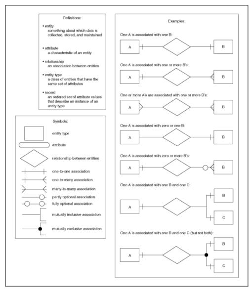
Figure 8–1 Rule for Drawing an E-R Diagram
