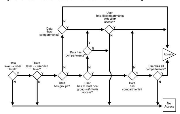
Figure 3–10 Label Evaluation Process for Write Access with COMPACCESS Privilege
